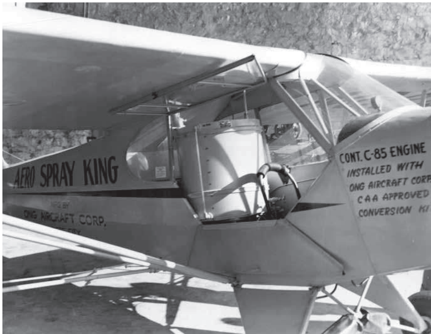
As sprayers developed new technologies, aircraft containment tanks continued to present a challenge. In the beginning, pilots designed their own chemical reservoirs by constructing a metal tank large enough to hold the necessary chemical loads and thick enough to resist corrosion. In later years, as agricultural aircraft standardized, tanks were double-lined to provide increased protection for applicators. Pictured is an Aero Spray King outfitted with a chemical tank, produced in the late 1940s by the Ong Aircraft Corporation of Kansas City.
