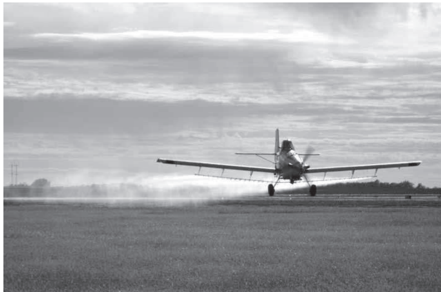
A spray pilot participates in a 2009 fly-in as part of Kansas State University's Operation SAFE in Salina, Kansas. The biannual event includes testing swath coverage by spraying colored dye on paper swatches located on the ground. Photograph courtesy of the author.
